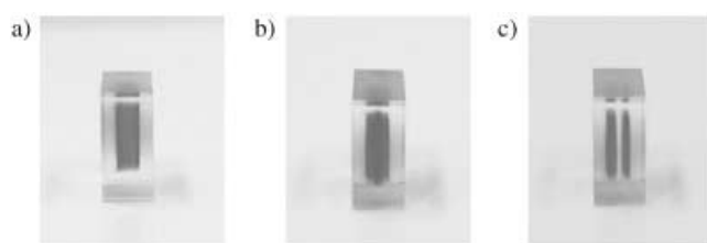
Figure 5. Photographs of images drawn inside the Au 2 O 3 -doped glass (0.01 mol %): a) by using femtosecond laser irradiation and annealing at 550 °C for 30 min; b) further irradiation at the center part of the image in (a) by focused femtosecond laser by using a 20× objective lens; c) then the glass was annealed at 300 °C for 300 min.
